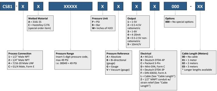
Ordering Example: CS81-2A00010PG4D000-00 (1/4" Male NPT, 316L SS, 0-10 PSI gauge, 4-20mA, Mini-DIN Form C)
