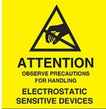
**ELECTROSTATIC DISCHARGE (ESD) Precaution** indicates user should take proper grounding precautions to prevent any potential damages from ESD.
